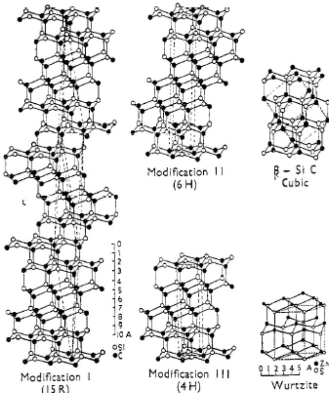
Fig. 1. The crystal structures of SiC (after H. Ott)
