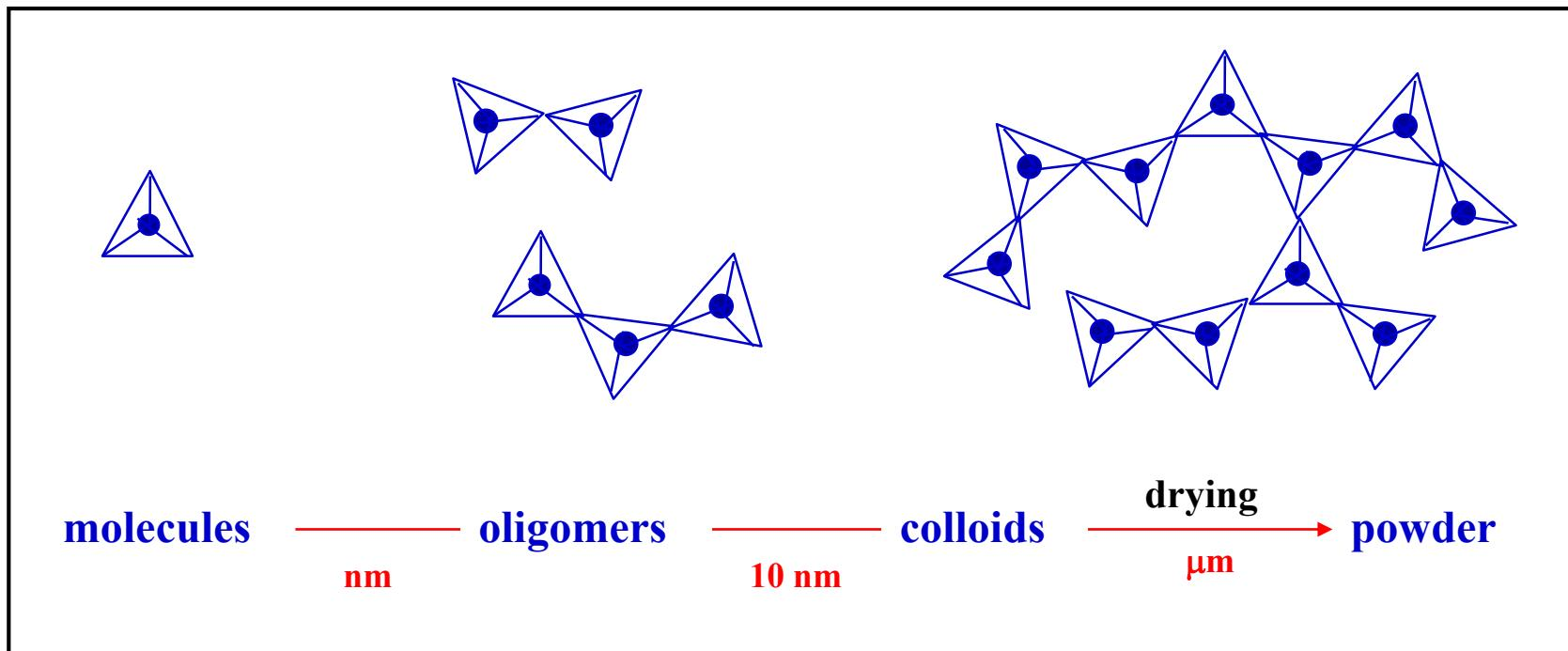
colloidal silica particles
