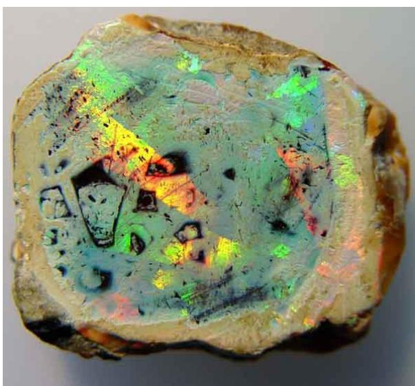
close-packed array of  $\text{SiO}_2$  spheres
