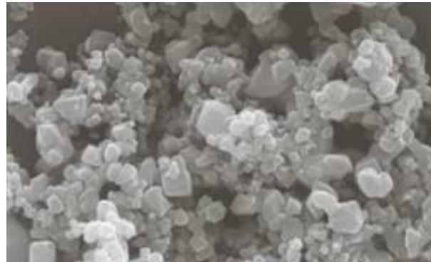
silica nanoparticles ( $\Phi \sim 15 - 500 \text{ nm}$ )
